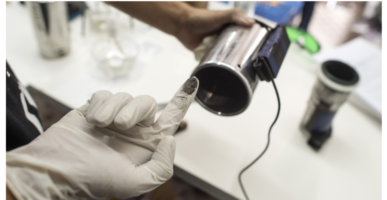
The mechanism used to capture the pollution in the form of soot called KAALINK.
